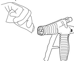
Change nozzles frequently! Foam will cure inside the nozzle in the same amount of time that foam becomes tack-free in the air.
