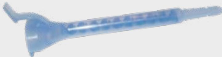
**ColorWise® Temperature Warning Nozzles** change from clear to blue, indicating that the chemical has reached cold temperatures below 60°F (16°C) and the foam should not be dispensed. Stop spraying to avoid off-ratio foam and yield-loss, and properly condition the chemical before spraying again.
