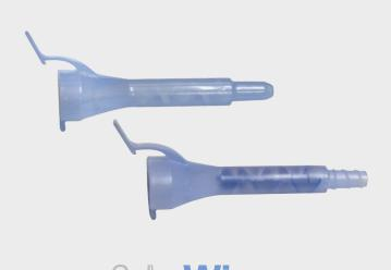
ColorWise® Temperature Warning Nozzles change from clear to blue, indicating that the chemical has reached cold temperatures below 60°F (16°C) and the foam should not be dispensed. Stop spraying to avoid off-ratio foam and yield-loss, and properly condition the chemical before spraying again.
