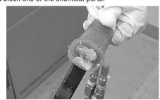
Change nozzles frequently! Foam will cure inside the nozzle in the same amount of time that foam becomes tack-free in the air.
