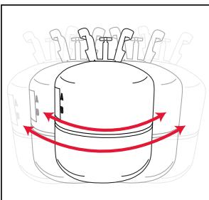
1. Shake each cylinder for 1–2 minutes before use to ensure proper mixing, see TDS for formula shaking and temperature recommendations on these instructions. Chemical should be between 70–85°F (21–29°C).
