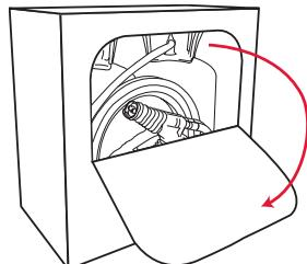
3. Push in top of front panel to open. Pull down flap for dispensing unit hose assembly. Remove nozzle packet and read instructions.
