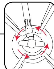
5. Open the valves completely by turning the valves COUNTER CLOCKWISE. Top flap may be removed or left in place during use or storage.
