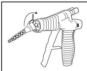
2. Insert bottom tab of nozzle into bottom slot of dispensing unit.
