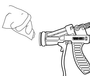
Change nozzles frequently! Foam will cure inside the nozzle in the same amount of time that foam becomes tack-free in the air.
