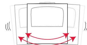
2. Shake kit for 1–2 minutes before use to ensure proper mixing. Typically chemical should be between 70–85°F (21–29°C). See TDS for formula shaking and temperature recommendations.
