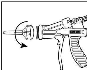
2. Attach nozzle by twisting to the right into the lock position.
