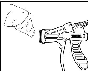
1. Before attaching nozzle, use petroleum jelly on face of gun.
