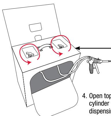
4. Open top flap of box to expose cylinder valves. Extend attached dispensing unit hose assembly.
