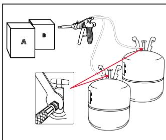
2. Thread red coded hose to A-component cylinder and black coded hose to B-component cylinder and tighten with supplied 9/16" wrench.
