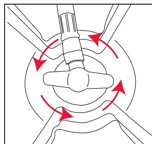
3. Open the valves completely by turning the valves COUNTER CLOCKWISE. Cylinder valves must be upright during use.
