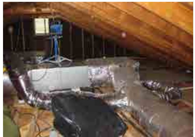
Ventilation testing set-up for spraying the attic floor
